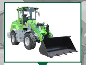
GEL-1800 Lithium 1.8T Electric Front Loader
