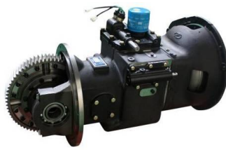
Transmission for forklift truck
